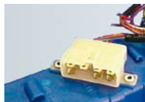
Automotive plastic connector to moulded chassis
